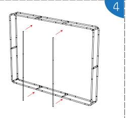
Install the middle tube to finish the frame
